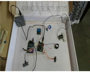
Whenever a threat is detected, that is ,any trespassing occurs a message is received at the end where security officials are located and further action is taken. In the above given setup we have used a mobile handset. The threats occurred are detected by the GSM.
